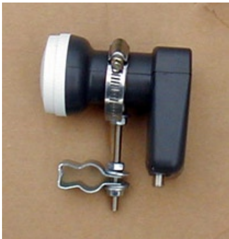
Fig 7: Ku-band LNB with adaptor can be mounted on a multi-feed holder to receive two Ku-band satellites on one dish. (Courtesy: global-cm.net)
