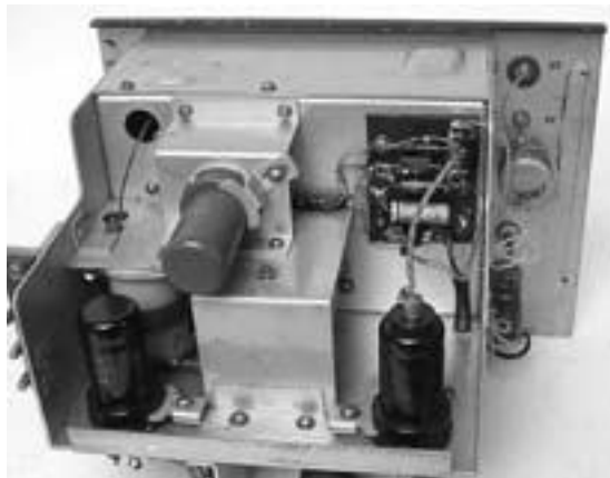
Top of the BC-221-AL chassis. Tubes are (from left), 6SJ7 audio output, ruggedized 6SJ7VFO, 6K8 oscillator/mixer.
