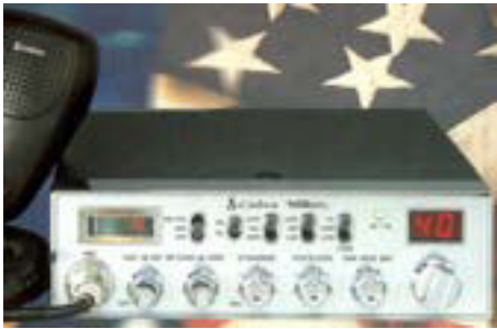
Cobra's 148GTL is one of a few models to offer AM as well as upper and lower sideband transmissions, but no NOAA WX channels. Retail for $155 at Universal Radio. (Courtesy: Universal-Radio)
