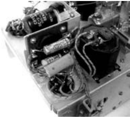
View of bottom of instrument. Paper capacitor marked "Tobe" and electrolytic with "+" marking are "rogue" parts. Behind them is the calibration crystal, which is on a metal tube housing.
