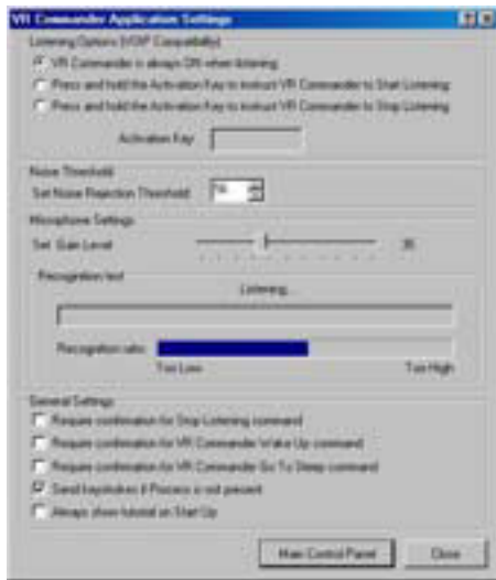
Figure 3 Checking for the proper microphone level
