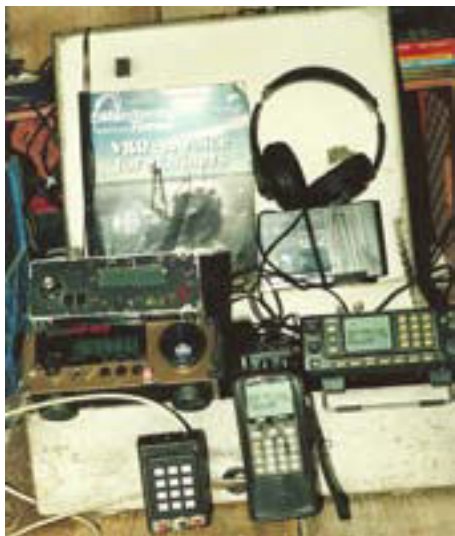
Present onboard set-up in old galvanized first-aid box, with HF150, MFJ Reader. AR8600 and 8200III on common antenna/preamp.
