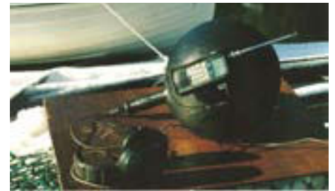
The Bionic Ear with AR8200III mounted on rear with headset with two sets of drivers/speakers.
