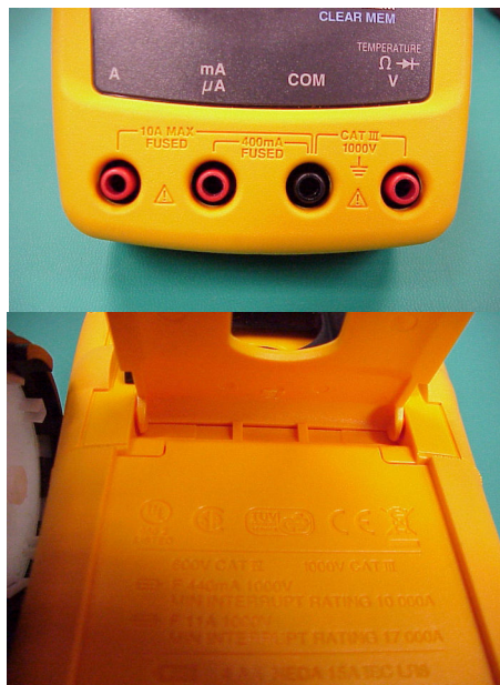
A good quality test meter that has safety agency approvals (UL/CSA)
