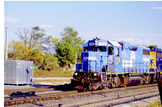
After the switch was functioning again and the CSX train was able to get a signal to proceed, it passes the sign marking D&S Junction. Behind the sign is the metal housing for the logic and safety circuits controlling the junction.
