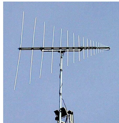
Create vertical log periodic dipole array may be the best VHF-DX antenna on the market. But, at $300 it had better be! (Courtesy: Grove Enterprise)
