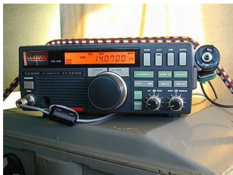
N4GVA's on-board digital station consisting of a Yaesu FT-747GX with a data/mic switch box and aviation headset interface for voice. (Courtesy: Scott Keating)
