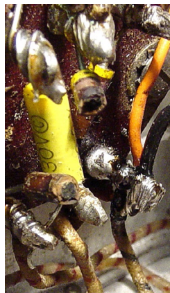
The two ends of the burned resistor after I fished them out from behind one of my replacement capacitors.
