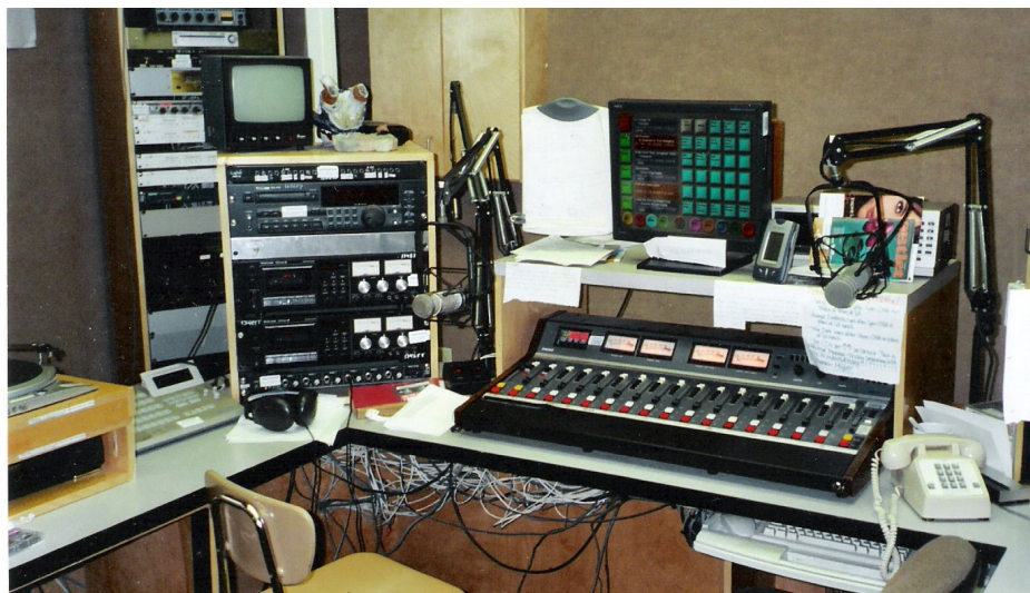
WFOS-FM main control room can broadcast from any source analog or digital, even 78 rpm discs. The computer screen above the console links the DJ to the station's Scott Automation 18.2 GB hard drive and the 8,000 song library via touch screen.
