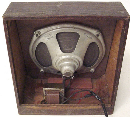
Speaker and output transformer in small tabletop baffle – all scrounged from junkbox. The baffle will get a coat of black paint to match the radio.
