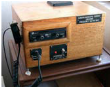
An old aircraft transceiver fitted nicely into a hand-crafted cabinet serves well as the Auburn Municipal Airport (AUN) UNICOM radio on 122.7 MHz.
