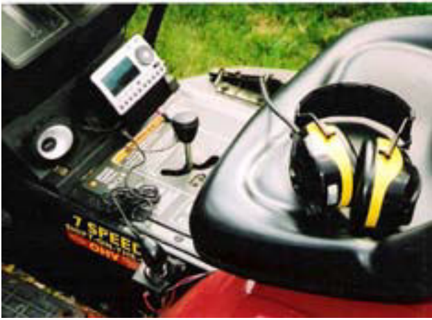
Tiny, magnetic mount XM satellite radio antenna mounts easily to the metal engine cover on the lawn tractor. A mag/mount 2 meter whip or scanner antenna would mount as easily and feed your HT or scanner. You can transmit the audio output to a small FM modulator and listen on a noise suppression headset. (Courtesy: Author)
