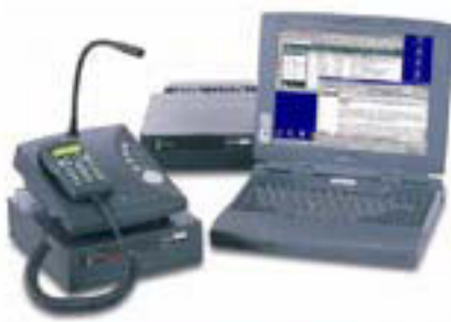
3012 HF Data Modem, NCT desk console, NCT RF Unit and computer
