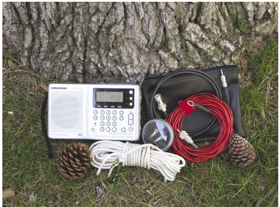
A complete station including a small portable radio with homemade FlexTenna, antenna adapter cable, antenna rope, and roll up earphones packs up easily into small pouches. Pine cones optional!
