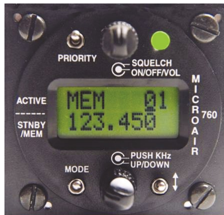
Microair M760 VHF Airband Transceiver. Do VHF aircraft transceivers receiver better than good scanners? Photo courtesy Microair Avionics.
