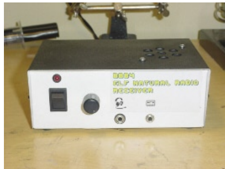
Figure 2. Tom Severt (KS) built this Natural Radio Receiver based on plans from the February and March issues of Below 500 kHz .
