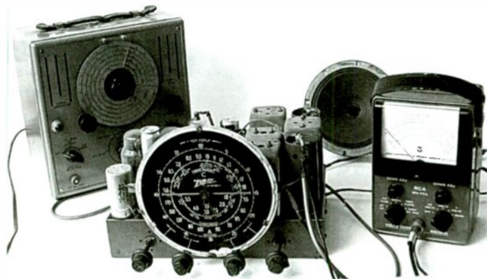
Alignment instruments included my trusty Triplet 2432 r.f. oscillator and RCA Voltomyst Jr. VTVM – both of which were rehabbed in previous “Radio Restorations” columns.
