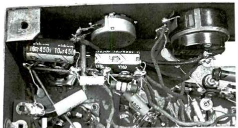
Newly-instelled terminal strip (at upper left) holds the two replacement electrolytic caps and also provides a tie point to substitute for one that "disappeared" (see text). Volume and tone controls are at top of picture.
