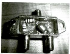
Fig. 4b: Diplexer with addition of 0.01 uF cap and split chokes
