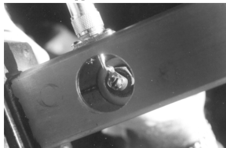
2. The coax connector centerpost is soldered to the antenna terminal spade connector.
