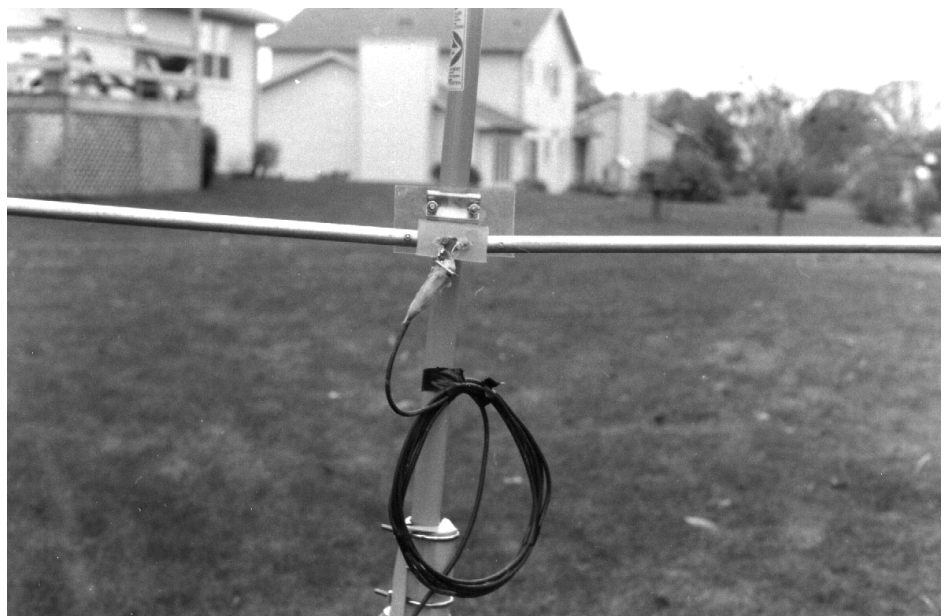
B. The lower section of the antenna is split into two parts to form a feed point for 52-ohm cable. A coil of coax cable provides a balun transformer to make an unbalanced feedline work with a balanced loop, as described in the text.
