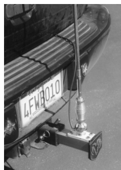
5. The RG-8U coax is fed to the antenna through the seal in the rear cargo door.
