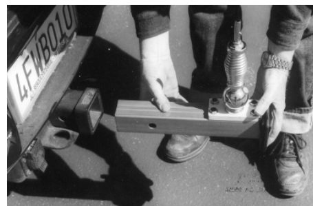
7. By pulling out the lock pin, the unit can be easily removed when not in use.
