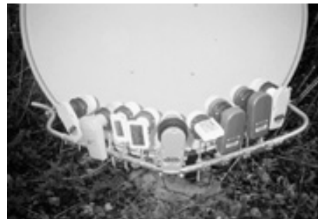
Multiple feeds allow one dish to "see" several satellites at the same time without moving the dish. (Courtesy: Global Communications)
