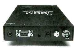
FIGURE 1 - IC-PCR1000 Back Panel
