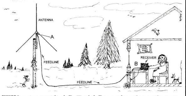
FIGURE 1: an antenna connected to a feedline (A), and a feedline connected to a receiver antenna-input connector (B).
