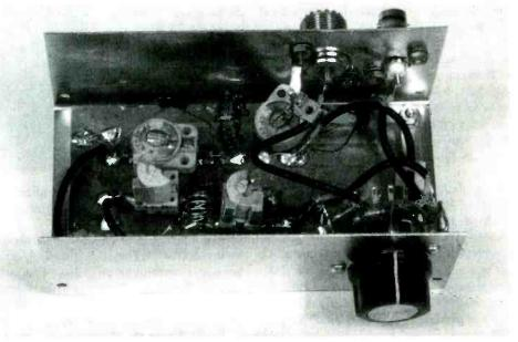
The matching circuits are built into a small aluminum box. The circuits themselves are tack soldered on a "universal" circuit board. In this design, three positions are provided: CB, 146-MHz ham, and scanner.
