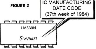
Examine the IC manufacturing date to help determine equipment manufacture date.
