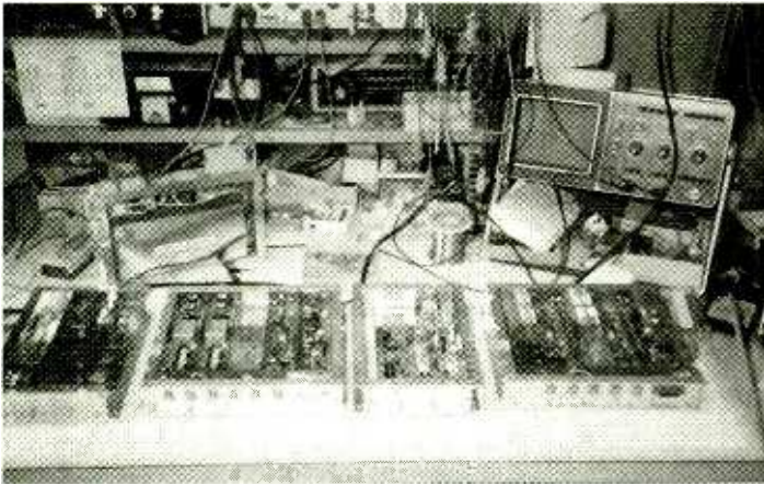
Some flight electronic modules for the Phase 3D undergoing final bench testing at the AMSAT-DL laboratory in Marburg, Germany, prior to shipment to Orlando, Florida, for integration into the satellite. (Courtesy Keith Baker KB1SF)
