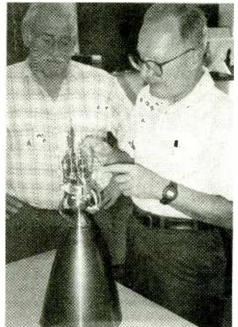
AMSAT-NA Vice President for Engineering, Dick Jansson, WD4FAB (right), and AMSAT-DL's Konrad Mueller, DG7FDQ (left), perform final inspection of Phase 3D's 400 Newton kick motor in Konrad's well-equipped machine shop in Germany prior to shipment to Orlando for integration into the satellite. The motor is the same design that successfully powered both AO-10 and AO-13 to their final orbits. Phase 3D will have a highly elliptical "molniya" style orbit allowing long contacts from across continents. (Courtesy Keith Baker, KB1SF)
