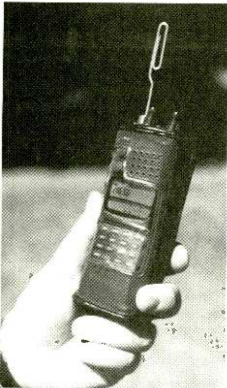
A bent paper clip can be used to short out the antenna lead, allowing the receiver case to become very sensitive to signal strength and direction.
