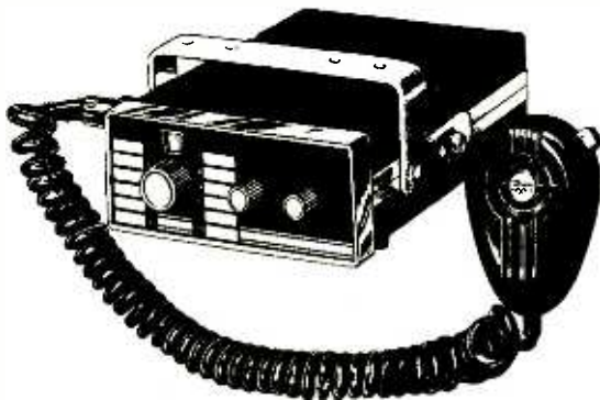
Fine old crystal controlled receivers such as this Regency unit are an inexpensive route to two-meters.
