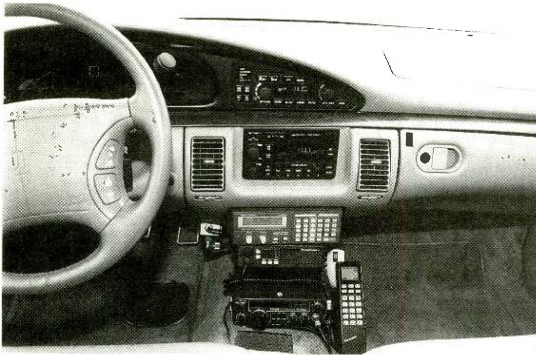
Armed with his PRO-2006 scanner, Motorola Radius UHF scanning transceiver, ICOM 255-A two meter transceiver, and a cellular telephone, the author is prepared for his next adventure in DFing. (Antenna switch to left of PRO-2006.)
