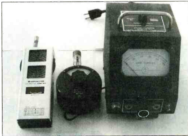
FIGURE 1 — This photograph shows two commercially made dip meters. The larger unit is a tube type, laboratory-grade instrument that was once produced by Measurements Corp. It operates from 1.6 through 420 MHz. The smaller solid state Kenwood unit is a DM-81 that covers the range from 1.6 MHz to 250 MHz.
