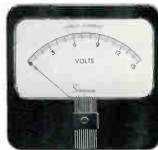
MODELS 29, 39, 49, 59 4 1/2" RECTANGULAR CASE. Width 4 21/32"; height, 4 13/64". Mounts in round hole. Body diameter 2 3/4". Scale length 3 29/32". Bakelite case.
