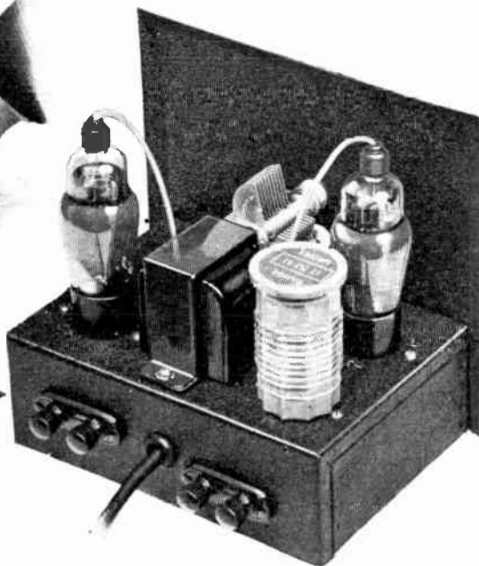
Mount tubes, tuning condenser, transformer, and plug-in coil atop the chassis; other ports below it
