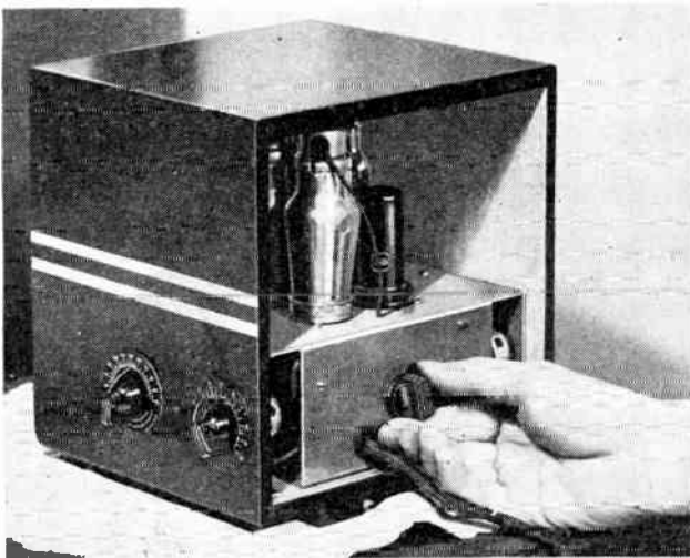
The chassis is placed well to the rear of the cabinet, to leave room for the speaker mounted behind the front panel
