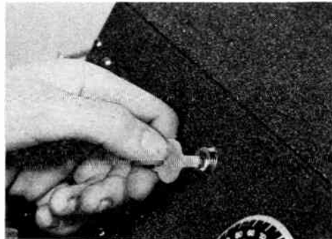
The antenna rod is set in a ceramic insulator atop the cabinet. Right, a key turns on the set
