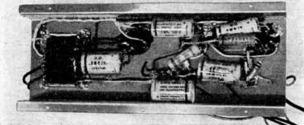
Top and bottom views of the amplifier chassis which should be bolted to the bottom of the suitcase under the motor-panel grill. Metal tubes are used—an important advantage in portable units
