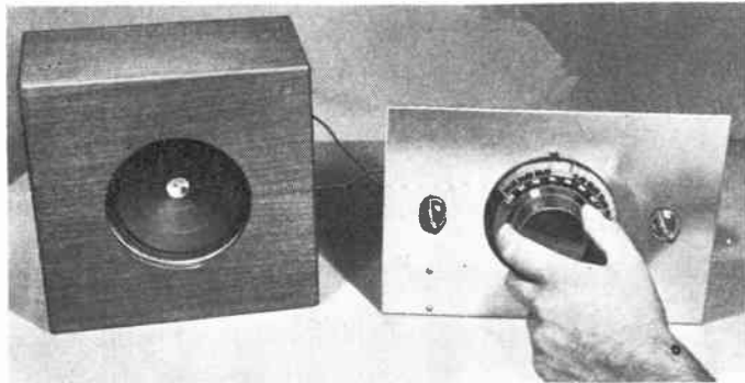
The circuit as it appears wired as a "four-tube" receiver. The antenna wire is coiled on the left. The clips at the right are for the speaker
