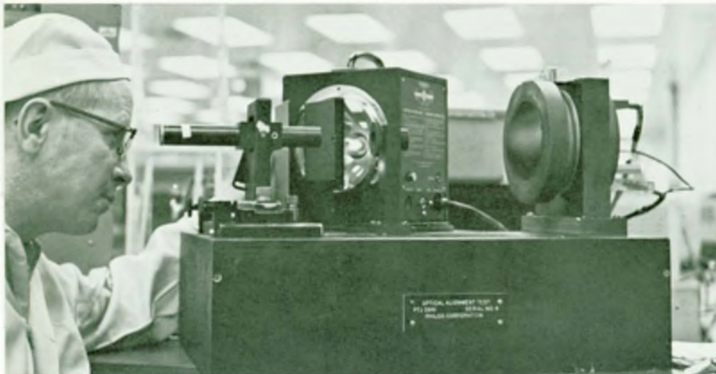
An alignment test for Sidewinder optics
