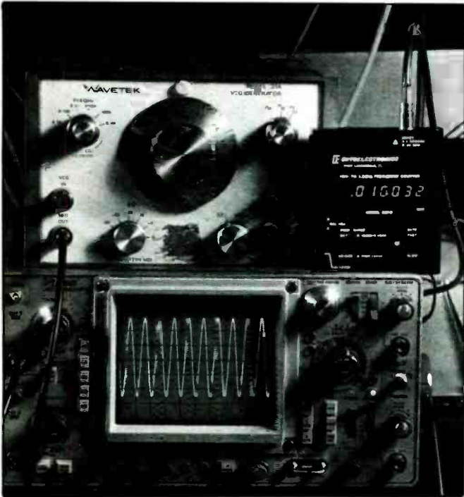
Direct Cable. Directly connecting a frequency counter to an oscilloscope's vertical channel output jack at the rear verifies a 1-kHz signal.
