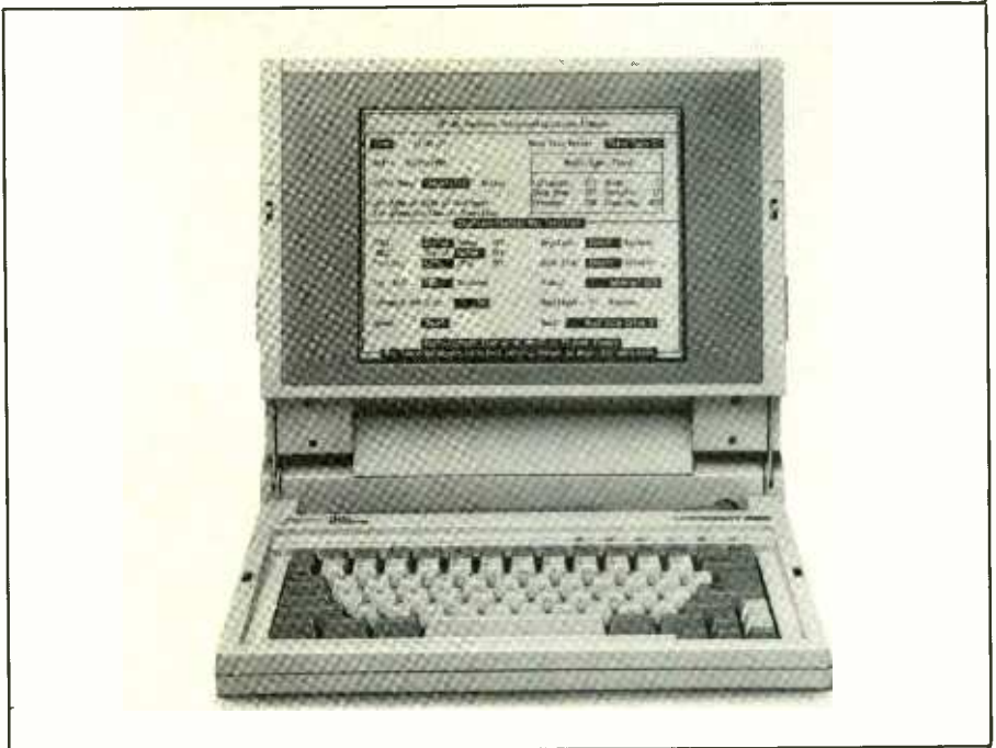
Zenith Data Systems' TurboPort 386 is a portable computer built around a 12-MHz 80386 processor, 2 megabytes of RAM and 20- or 40-megabyte hard disk. Though it can be operated on battery for about a half hour, it is not a true laptop computer.
