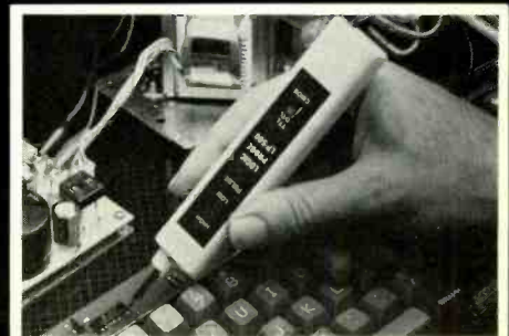
After you build this digital logic probe, you'll explore the operation of the Sanyo detached "intelligent" keyboard and its dedicated microprocessor.
