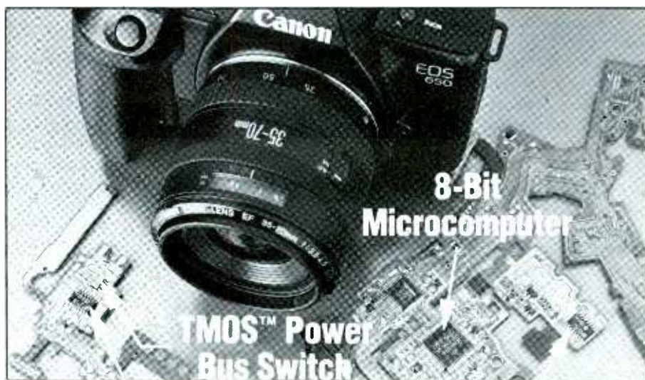
The innards of a new Canon 35mm camera reveals the important uses of electronic devices for photographic equipment. In this case, the various surface-mount devices highlighted are from Motorola's semiconductor sector in Phoenix.
