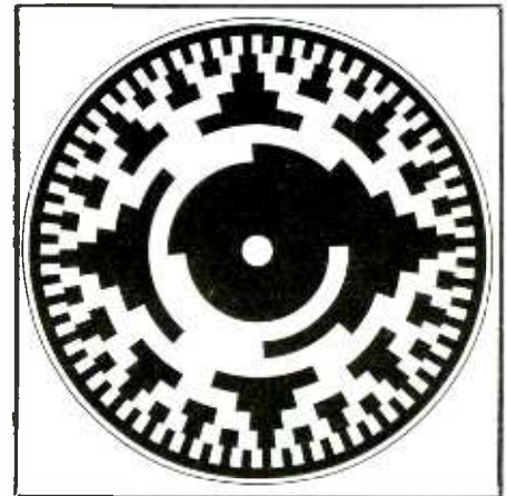
Fig. 2. An encoding disc for an absolute shaft encoder.
