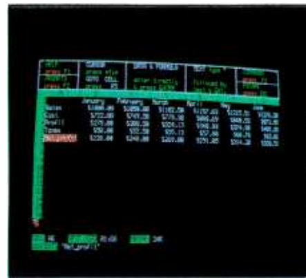
QL Spreadsheet is very powerful, yet easy to use. Here, only the value in cell "B" was input; all other values were then calculated from formulas.
