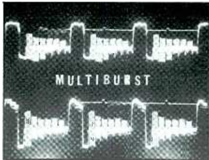
Computer I and II video inputs show full response but slight clipping.
