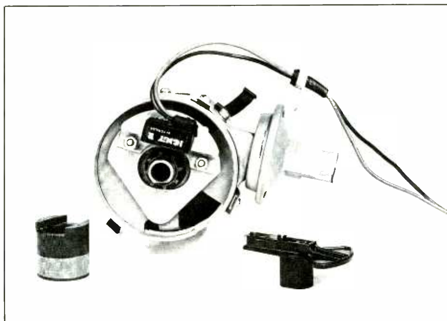
Fig. 2. Installation of the Ignitor kit begins with removal of the cap, rotor, points, and condenser from the distributor. The adaptor plates and solid-state ignition module are then installed in place of the stock parts as shown. Complete illustrated step-by-step instructions are provided in the kit to guide the do-it-yourselfer through the installation procedure.
