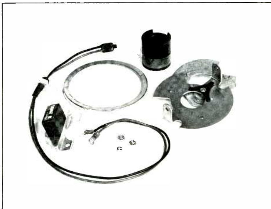
Fig. 1. One of the simplest retrofit electronic-ignition systems on the market, the Per-Lux Ignitor kit contains (clockwise from top) a magnet assembly, adaptor plates, a wiring harness and installation hardware, the Ignitor module, and a spacer for the distributor cap. The spacer plates may or may not be required, depending on the distributor in the vehicle.
