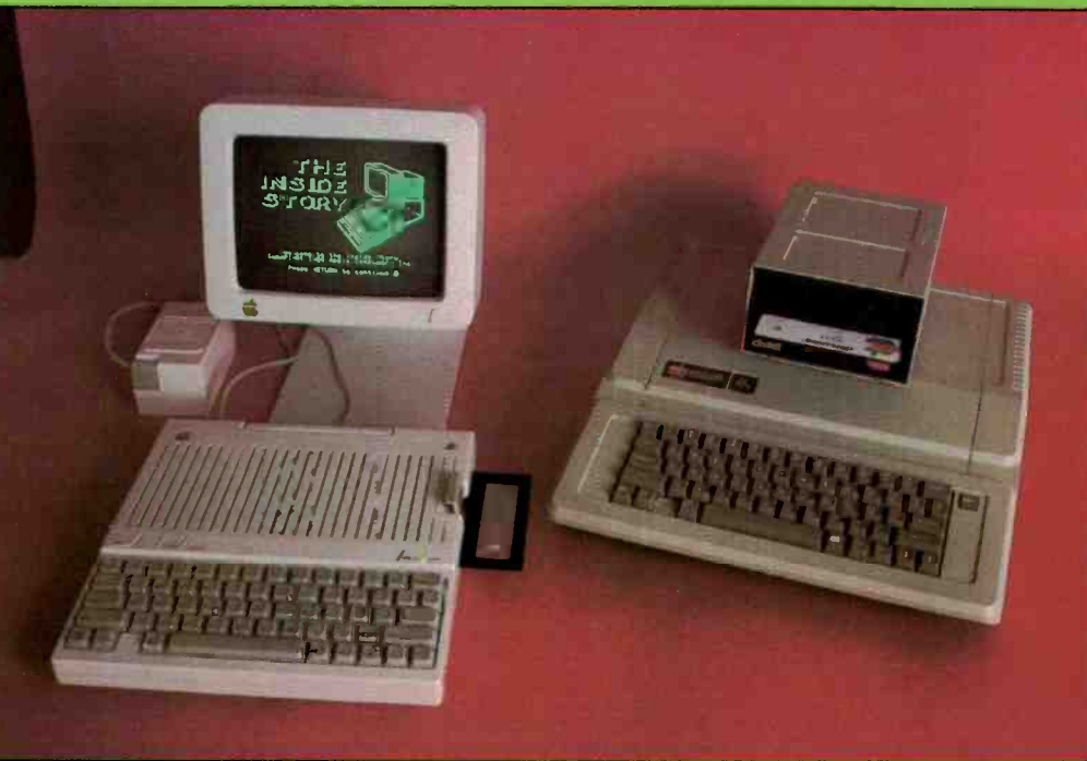
An Apple IIc at left, with its built-in disk drive and optional video monitor, is contrasted with an Apple IIe model with an external drive.
