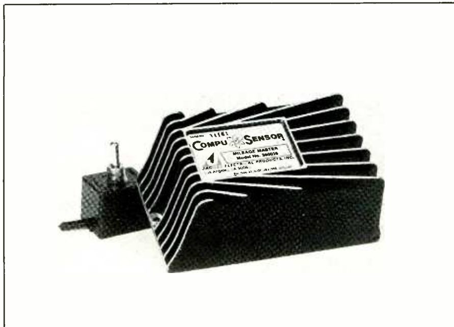
Jacobs Electrical brings the automobile into the computer age with its Compu Sensor ignition system. This unique device actually senses the resistance of each spark plug's gap prior to firing and then delivers a spark of proper energy and duration for each cylinder. The unit also features a three-position switch that enables the driver to turn it on for normal operation, off for ignition diagnosis and tuneups, and to disrupt the ignition system and serve as an anti-theft device.
