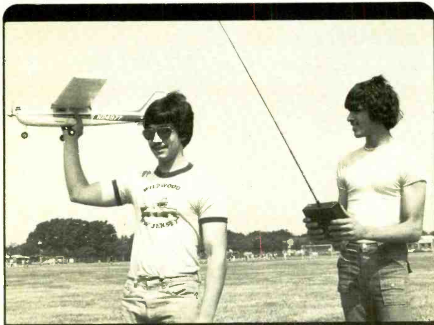
Charles Gianetto holds a Cox Cessna Centurian trainer while his brother Michael checks out the controls. The Cox Centurian comes almost ready to fly with its muffled engine installed, control push rods in place and provisions for the R/C receiver molding into the all-styrofoam interior. It's the ideal beginners plane.
