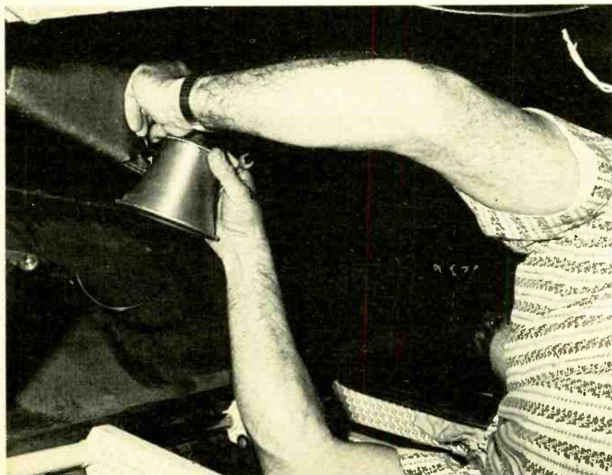
Under the deck, find a suitable mounting spot to attach the horn bracket. Hold the bracket in place, mark through the bracket holes, and drill. Secure the horn to its bracket with hardware provided, then run horn wiring to the alarm module. After all connections are made per directions the system is ready to work for you to protect your investment.
