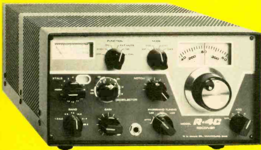
A ham bands only receiver such as this R.L. Drake R4-C gives you the kind of bandspread and sensitivity that makes receiving a pleasure. Front panel controls let you adjust the bandpass to custom tailor selectivity. A built-in notch that can drop out an interfering signal. The R4-C can be used as a transceiver with the addition of the T4-C transmitter.
