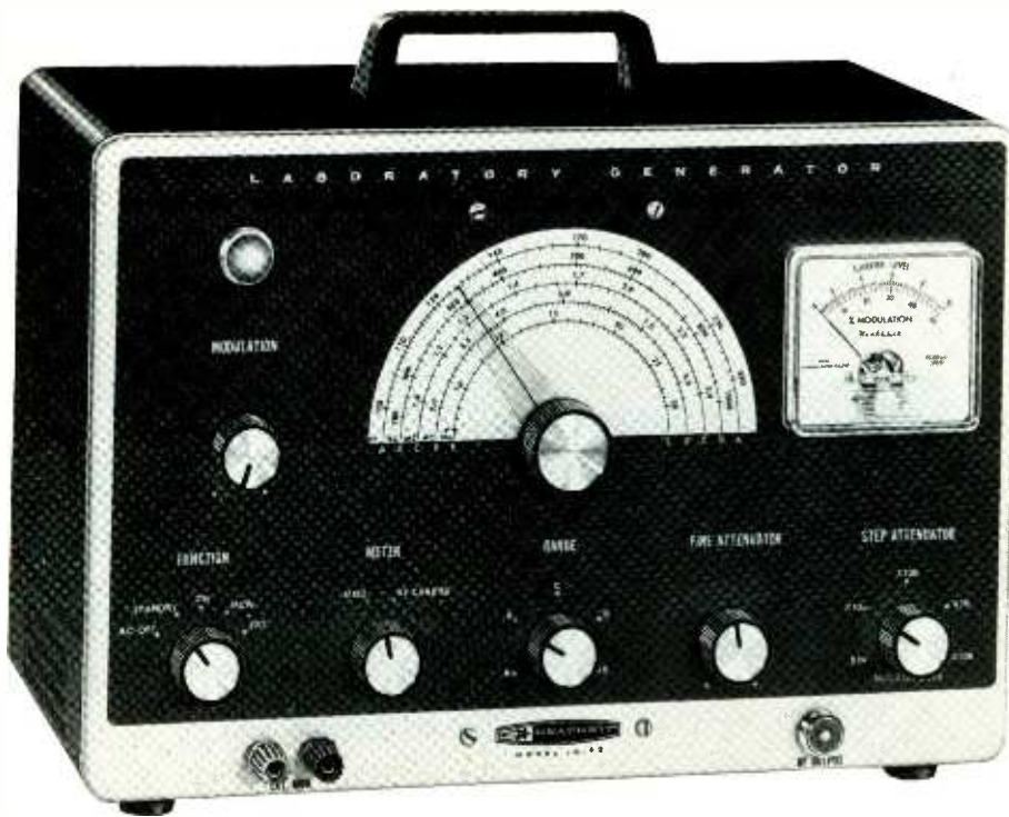
If you're into rf, you'll find an rf generator an absolute must. This Heathkit IG-42 is typical of most low-cost generators. You get the frequency by a combination of range switch and dial settings. The output level, which is monitored by an output meter, is adjusted with step and vernier attenuation controls. Another control lets you choose between a pure rf carrier or a carrier with amplitude modulation.
