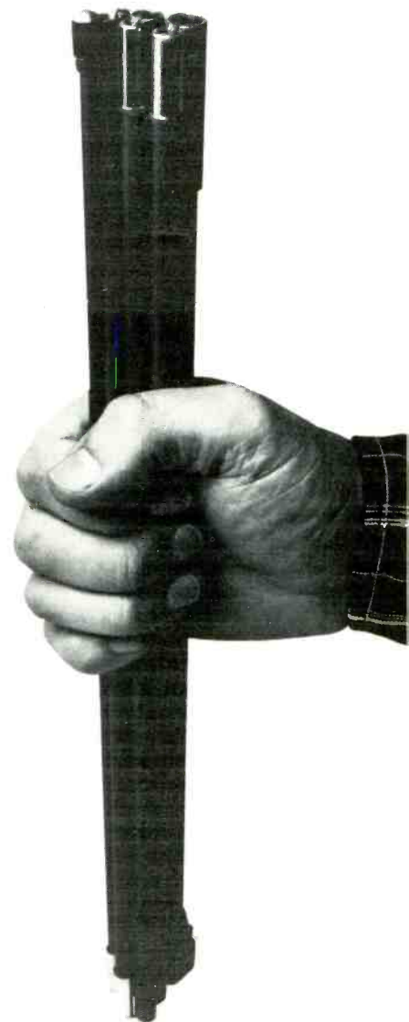
South Shore Trading Corporation offers a 102" whip that folds to a compact 15 \frac{1}{2} " in seconds. The SST Whie-A-Way antenna consists of a series of hollow, interlocking steel sections that are "strung" on a spring-loaded cable.
