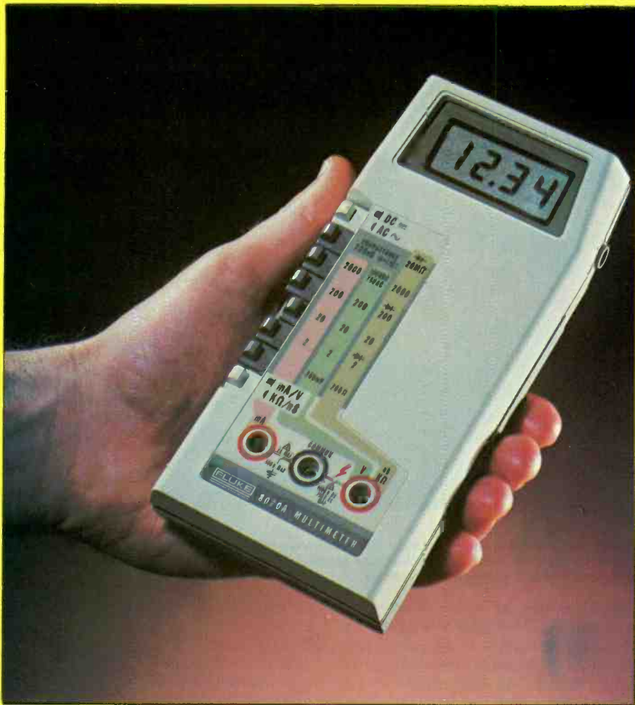
John Fluke's new hand-held digital multimeter is typical of the new generation of pocket-size instruments now available. This meter uses liquid crystal display readouts while most other hand-held multimeters use LEDs.
