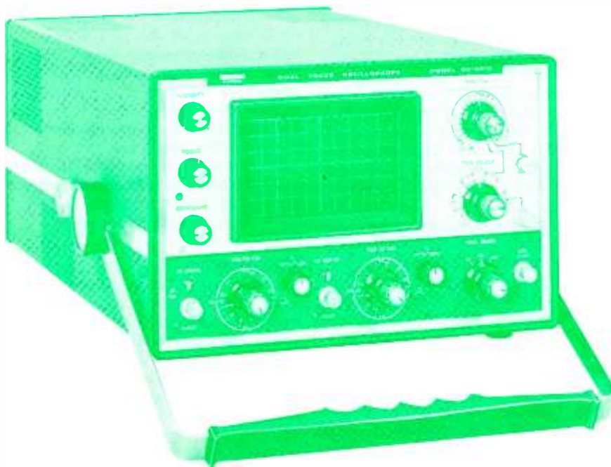
Figure 2 The Heath SO-4510 is typical of the sophisticated dual-trace scopes now in use. The simple layout and intelligently labeled controls make it easy to operate.
