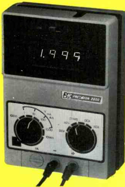
B&K Precision's portable DMM is this Model 2800. Except for the 3½-digit display, the 2800 is very similar in appearance to any small VOM.
