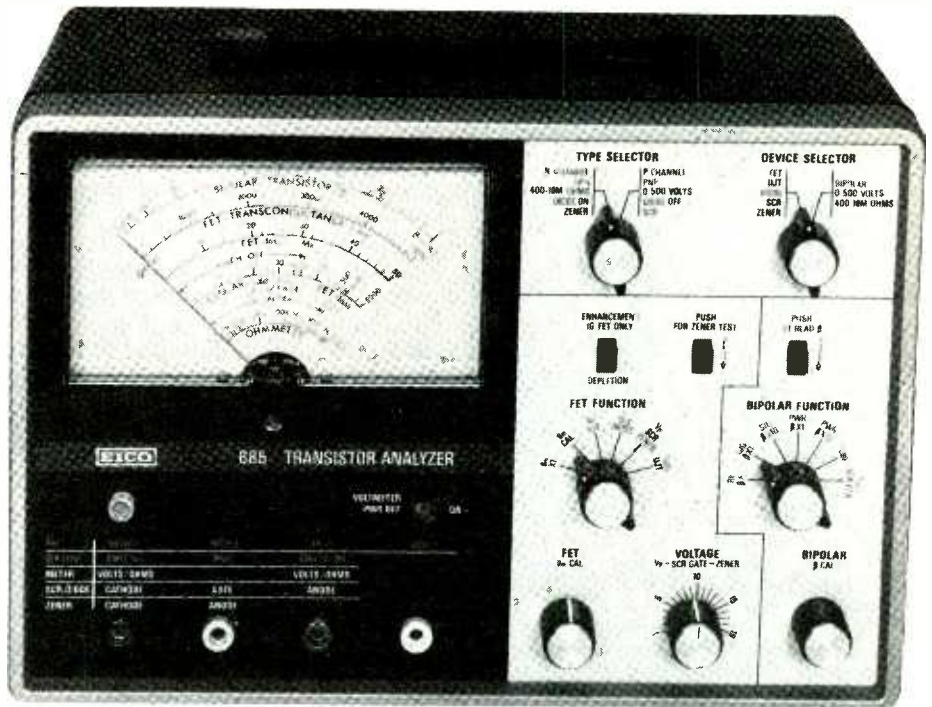
This Eico Model 685 is typical of the meter-type transistor tester. Although not as versatile as the curve tracer, most transistor testers can give you an accurate measurement of gain, and some gain-bandwidth product as well.
