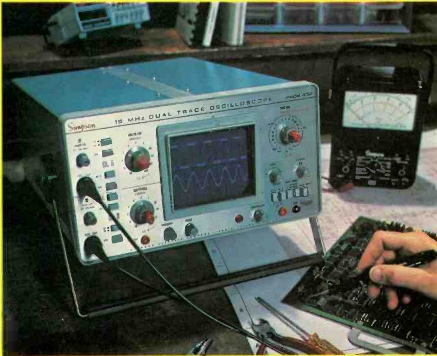
Oscilloscopes are unquestionably the most versatile piece of test gear you can own. Dual-trace scopes, such as this Simpson Model 452, let you compare amplitude, frequency and phase of two different waveforms.
