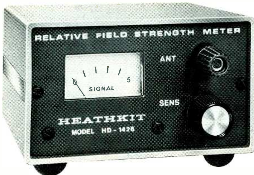
A relative field strength meter, such as this Heathkit HD-1426, is ideal for casually monitoring your transmitter and antenna system. Some field strength meters have built-in telescoping antennas. Others, including this Heath unit, require a length of hookup wire for the antenna.
