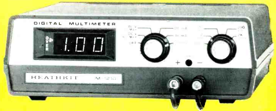
If you enjoy building your own gear, both Heathkit and Eico offer a variety of test equipment in kit form. This 2½-digit multimeter can measure voltage up to 1000 V, current up to 2 a, and resistance up to two megohms. In kit form, the price is $70; an assembled version costs $110.
