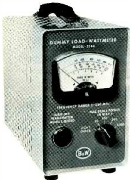
Dummy loads, such as this B&W Model 334A, let you run tests on transmitters under full operating conditions without having to worry about causing interference. Just connect it to the antenna terminal and it radiates the rf output in the form of harmless heat. This load will handle up to 1000 watts and has a built-in watt meter.
