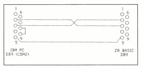
Fig. 4. Z8 BASIC to IBM PC serial interface cable wiring details.
