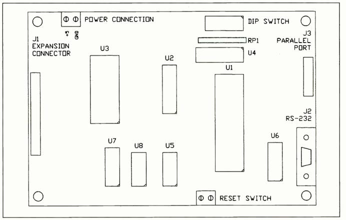
Fig. 2. Actual-size layout for components on perforated board that has holes on 0.1" centers.
