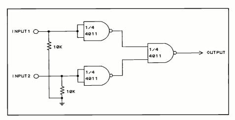
Fig. 1. Schematic details of a circuit you can use to have two devices share the same IRQ.
