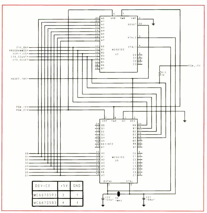
Fig. 1(C). Wiring details for Programmer's socket connectors.
