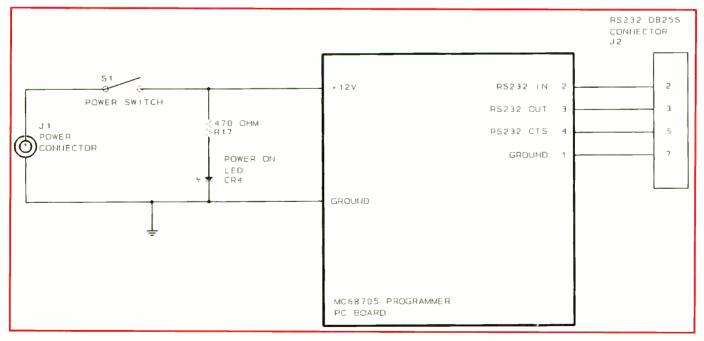
Fig. 5. Wiring details for power-switching/indicating and DB-25S connector circuits.
