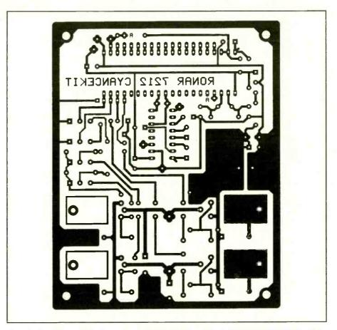
Fig. 2. Use this actual-size artwork for fabricating your own printed-circuit board on which to wire the motor-drive circuit.
