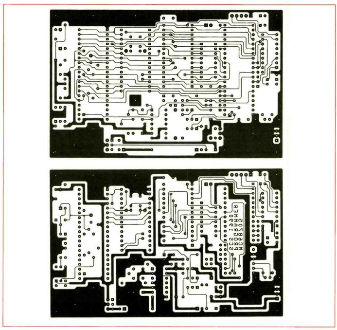
**Fig. 2.** Actual-size etching-and-drilling guides for Programmer's double-sided printed-circuit board. This board should have plated-through holes; otherwise, you must solder all connections on *both* sides of board and use short wire vias in areas where component leads/pins do not bridge from one side of board to other.
