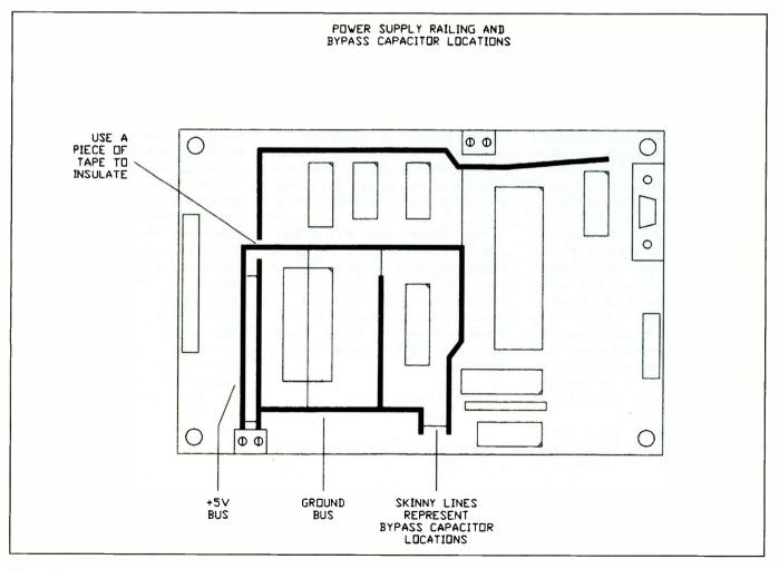
Fig. 3. Bottom view of board shows power-supply buses and locations of bypass capacitors.
