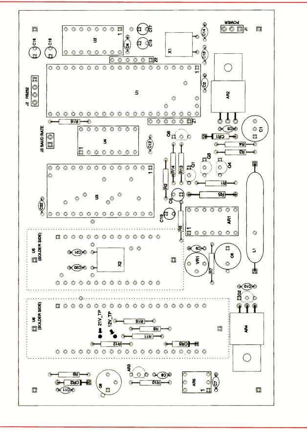
Fig. 3. Wiring guide for printed-circuit board. Note that ZIF sockets plug into standard solder-tail DIP sockets on solder side of board.
