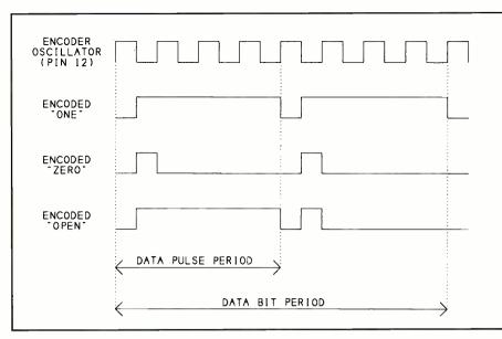
**Fig. 3.** The MC145026 trinary encoder outputs these pulse patterns to indicate logic 1, logic 0 and open-circuit conditions at its data and address inputs. Each bit requires eight oscillator cycles to transmit.
