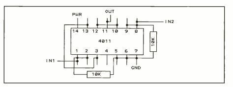
Fig. 2. Wiring details for the add-on IRQ-sharing circuit.
