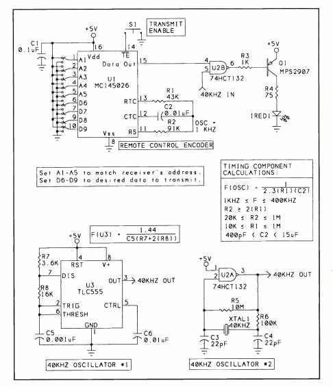
**Fig. 1.** This infrared transmitter sends four bits of data to a receiver identified by a five-bit address. Transmitted pulses are chopped at a 40-kHz rate. You can build a 40-kHz oscillator using a 555 timer or from a logic gate and 40-kHz crystal.
