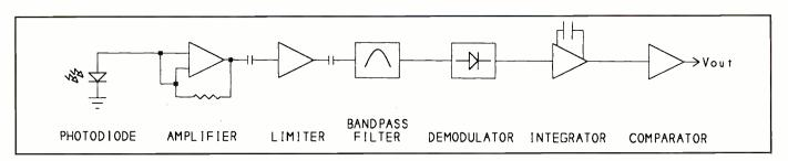
Fig. 4. The GP1U52X infrared receiver module is a detector, amplifier and filter in a three-pin package. When the module detects infrared energy pulsed at 40 kHz, Vout goes low.
