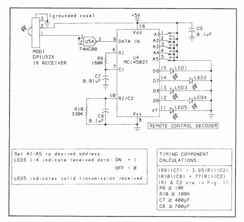
**Fig. 2.** This infrared receiver identifies transmissions intended for it and makes the received data available at D6 through D9.
