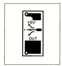
Fig. 4. Actual-size artwork for Hall-effect sensor assembly.
