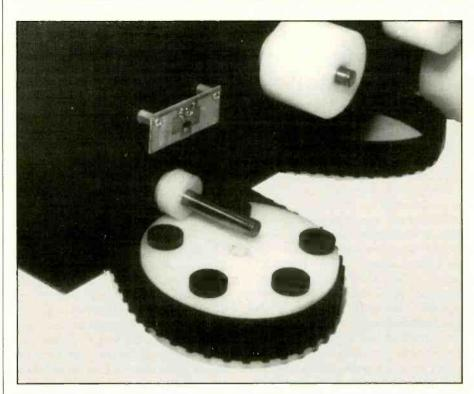
Magnets mounted in holes in drive wheels trip Hall-effect sensor on small pc board located just above wheel axle.
