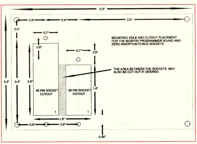
Fig. 4. Socket/pc-board mounting template.
