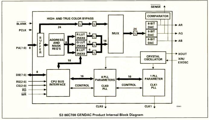
Fig. 1. Integrated Circuit Systems' and S3's GENDAC chip offers flexibility with its dual independently programmable pixel and memory clock outputs.
