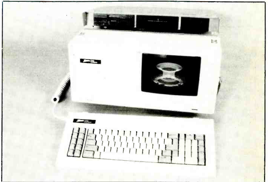
Heath/Zenith Z-160 flip-top transportable IBM-compatible computer is one of two candidates for upgrading as described in this article.
