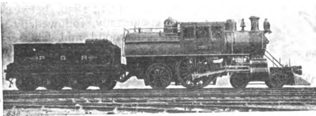
THE BICYCLE TYPE LOCOMOTIVE WHICH WAS DESIGNED FOR HIGH SPEEDS AND WAS THE FORE-RUNNER OF THE ATLANTIC AND PACIFIC DESIGNS
