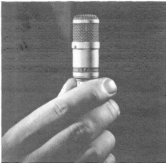
Figure 11—This miniature capacitor microphone, containing a transistor amplifier in the case, is designed for television broadcasting.
