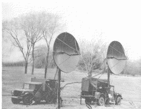
Figure 19—The AN/TRC-112 may be set up for operation within a half hour after reaching a site. The entire equipment is stowed in the two trucks for transportation and two small trailers (not shown) carry the primary power source.
