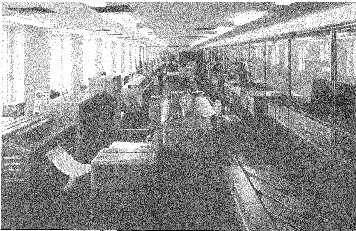
Figure 6—View of trial installation. The envelope stuffer and line printer are at left foreground and the stamping device for sealed letters is at right foreground. The document sorter equipped with 12 pockets and the reader-sorter equipped with 17 pockets are in the background.
