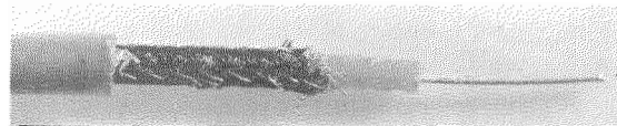
Figure 22—Miniature coaxial cable insulated with carbathene. On soldering the conductors there is no run-back of the insulation.
