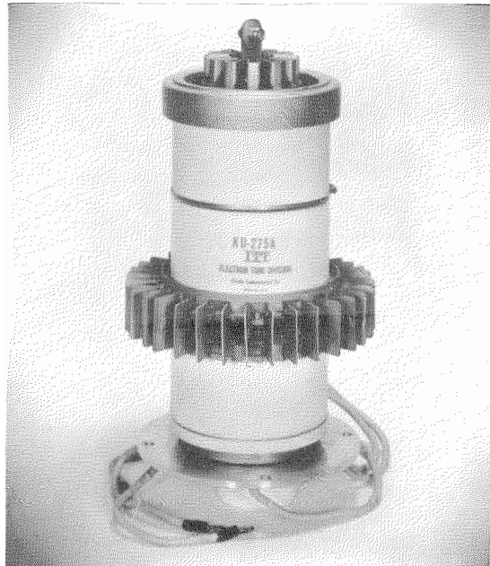
Figure 9—Ceramic-insulated thyatron capable of controlling a peak power of 100 megawatts.
