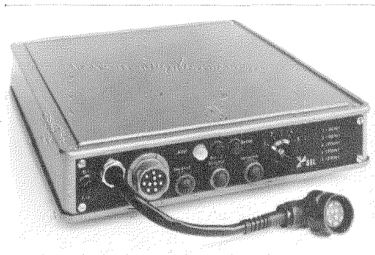
Figure 16—Fully electronic selective call unit for mobile radiotelephone networks. As many as 1980 separate stations may be called individually.
