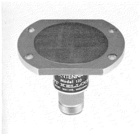
Figure 17—Double-spiral antenna for 2.5 to 11 gigahertz. This receiving unit is only 2.5 inches (6.3 centimeters) in diameter.
