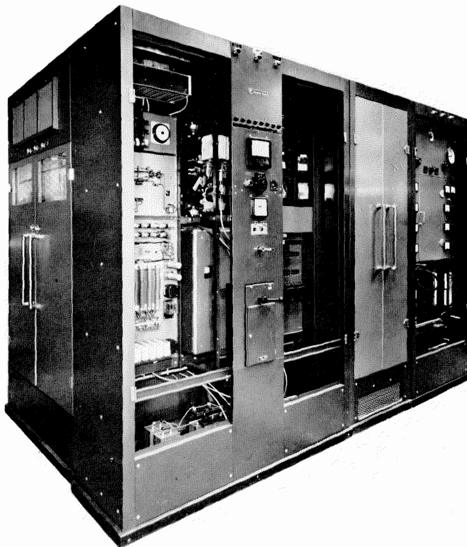
Figure 1—Ten-kilowatt transmitter. The power control unit occupies the two open bays at the left, the transmitter drive is next, and at the right end is the klystron cabinet. Behind the power and drive units, with its panel showing at the extreme left, is the extra-high-tension cabinet.
