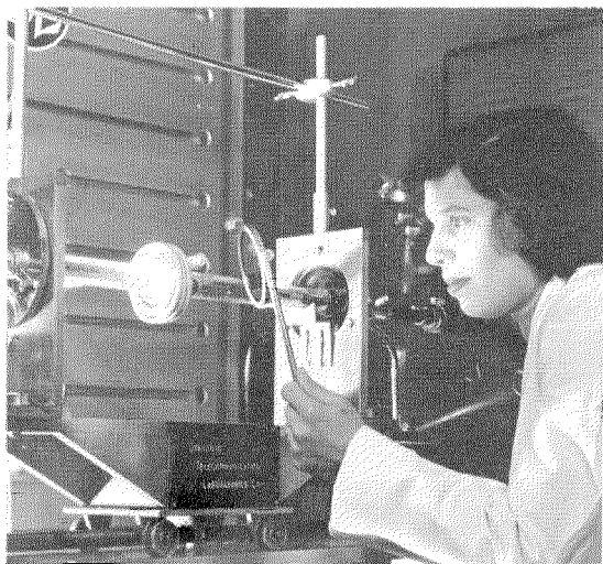
Figure 11—Localized radio-frequency heating is used in zone refining of material held in a water-cooled silver crucible.
