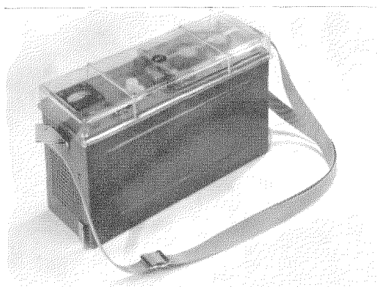
Figure 4—Portable tape recorder using cartridge magazine for tape storage. The transparent cover permits use in inclement weather.
