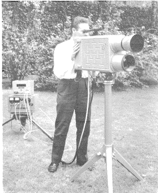
Figure 6—Range finder operating on a single pulse from a ruby laser.
