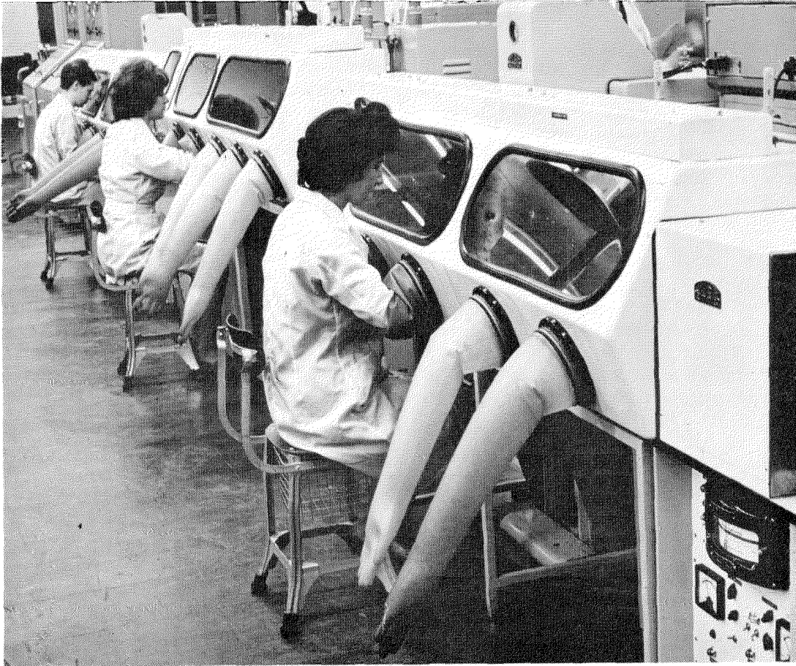
Figure 3—Cabinets providing small, clean, temperature-and-humidity-controlled enclosures in which transistors are encapsulated.
