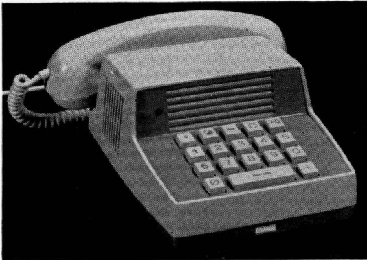
Figure 3—Intercommunication set having both handset and loudspeaker for connection to a private automatic exchange. The 5 buttons in the top row are for direct selection, camp-on-busy, transfer, staff locator, and loudspeaker. In the bottom row are buttons for microphone short-circuit, press-to-talk, and release.
