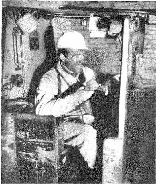
Figure 8—Mine locomotive operator speaking over the ZIG frequency-modulated carrier telephone system. The loudspeaker is permanently mounted above his shoulder.
