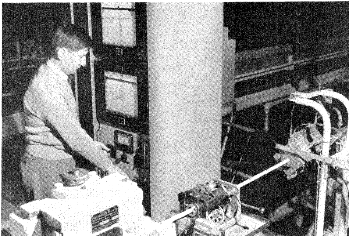
Figure 5—Take-up platform with recorders for diameter and capacitance per unit length of the core is at the cold end of the long cooling trough.
