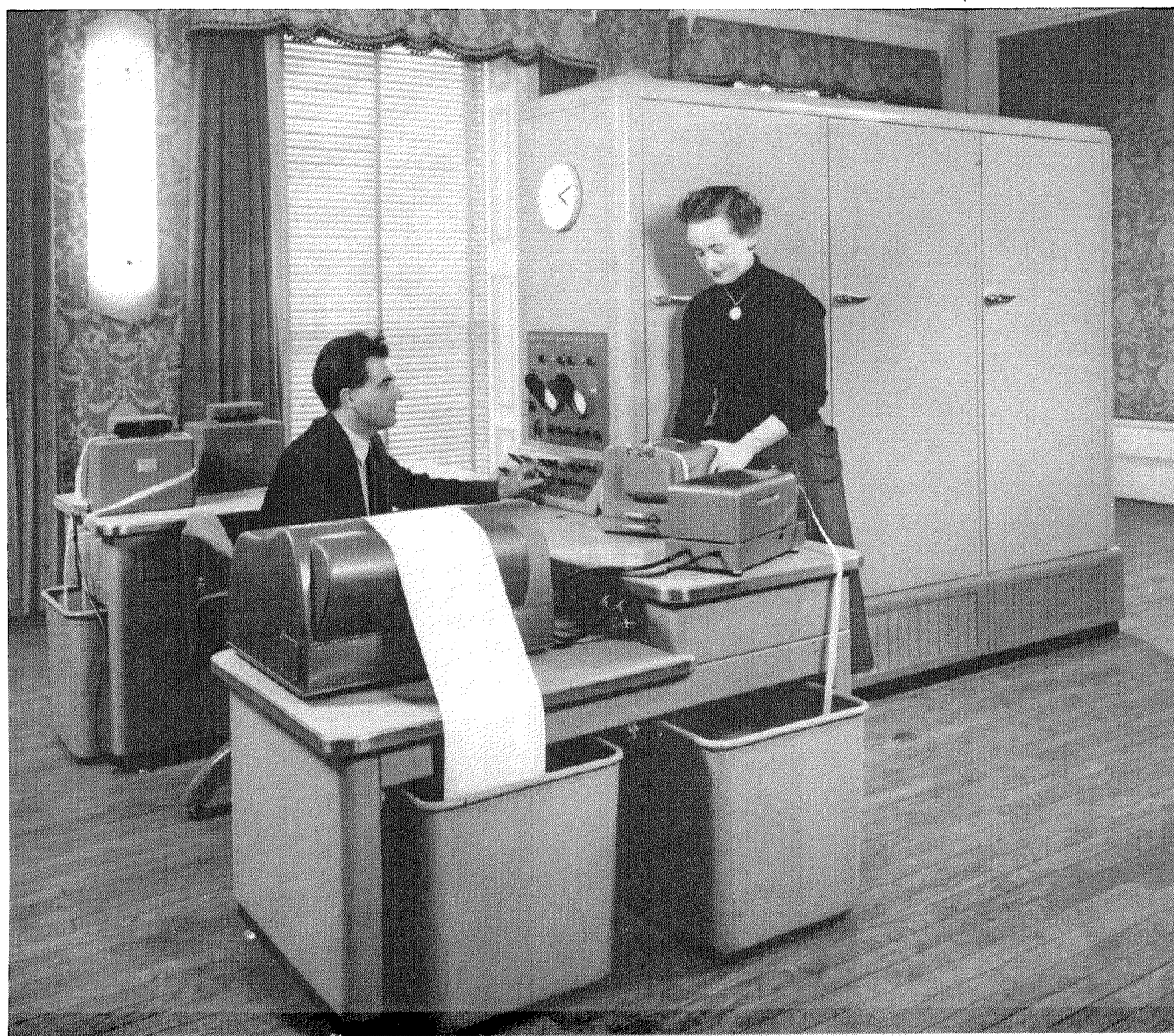
Figure 3—Application of teleprinter equipment to record output data from an electronic digital computer in punched-tape and printed-page form.
