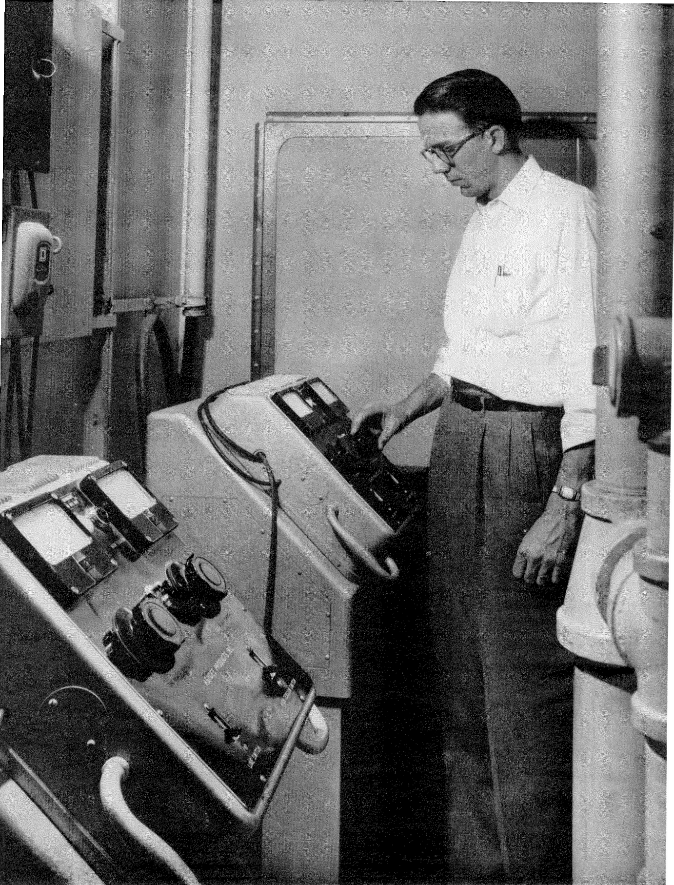
6. The author at the controls of one of the two 100,000-volt power packs that supply the electrostatic charge in the paint-spraying booths.
