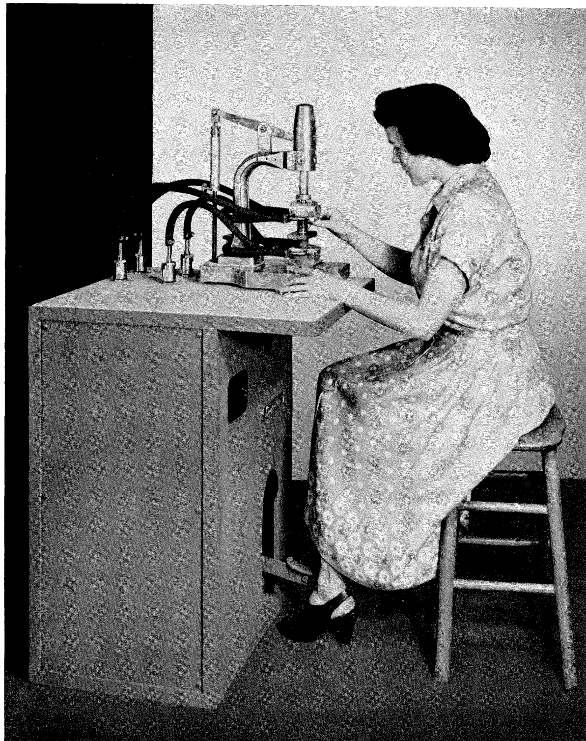
Figure 4—A production-line-type resistance brazing machine. On this 10-kilowatt equipment, the carbon electrodes are mounted in water-cooled holders. Pressure on the foot-pedal causes the electrodes to come together and grip the work firmly. The current is then applied until the brazing alloy melts; pressure is maintained while the work cools.
