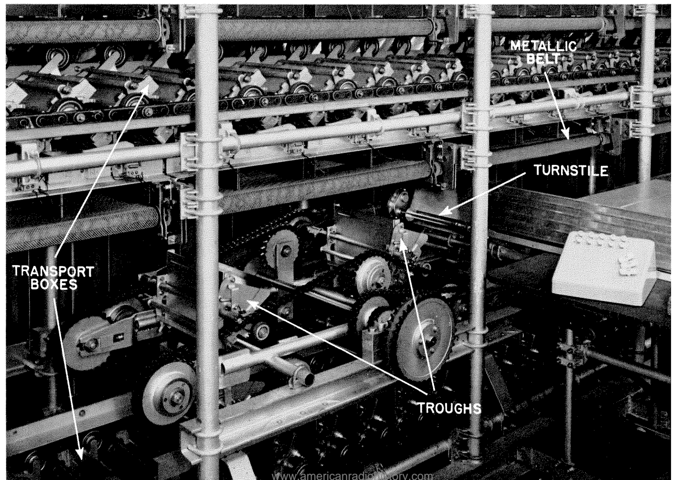
Figure 5—The troughs on the transfer device and some other parts of the machine are shown below.
