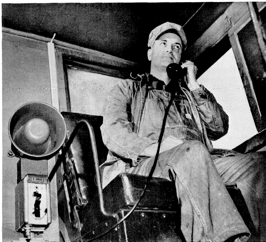
A freight-train conductor, while sitting in the cupola of his caboose, may speak by radiotelephone directly to the engineer of his train, to the crew of a passing train, or to the division dispatcher through the nearest way station.
