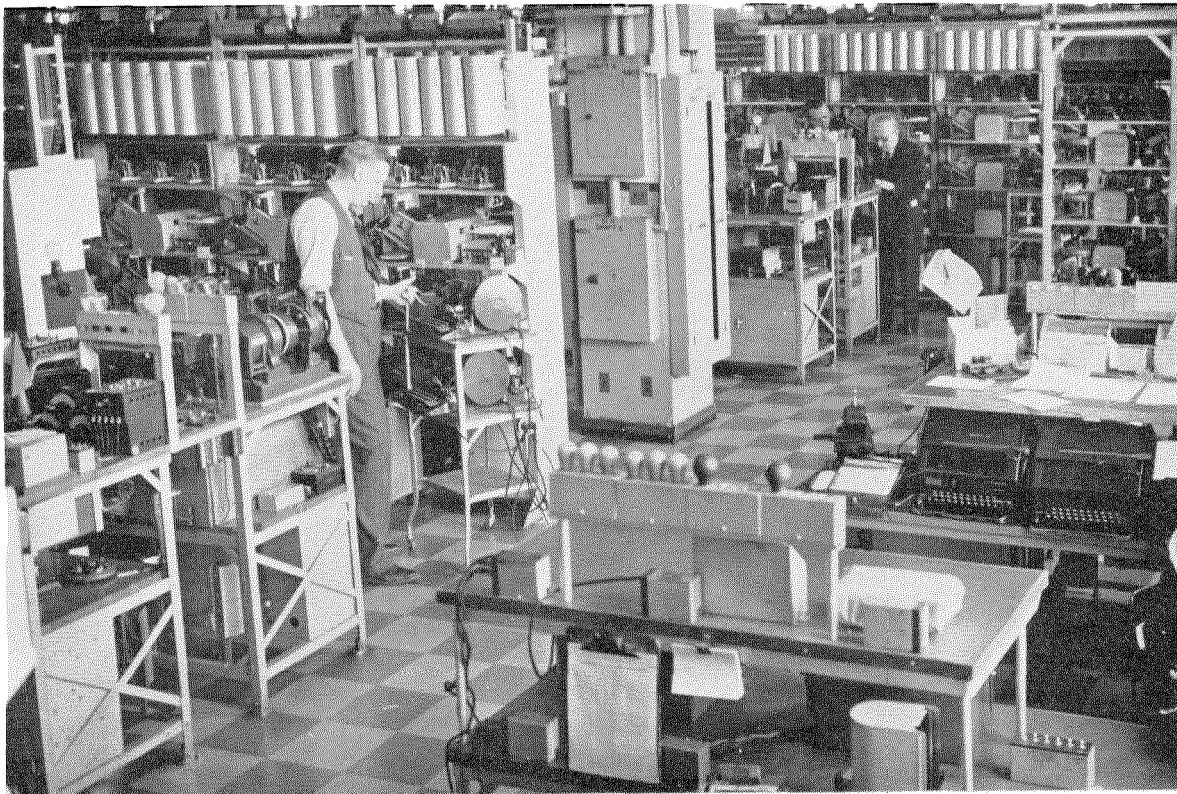
Fig. 2—Varioplex Central Office equipment.
