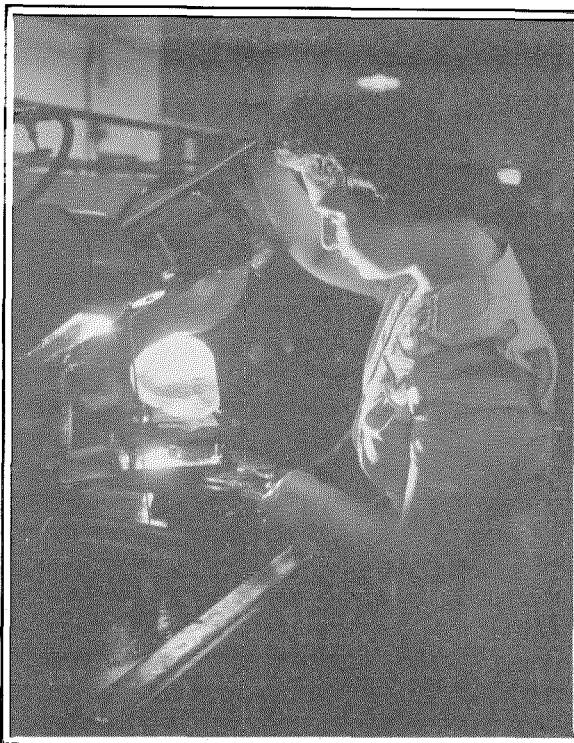
Fig. 8—Operator at the Federal Telephone and Radio Corporation Crystal Laboratories in Newark, New Jersey, Adjusting a High-Speed, Diamond-Impregnated Blade for the Initial Cutting Operation on a Piece of Raw Quartz.
