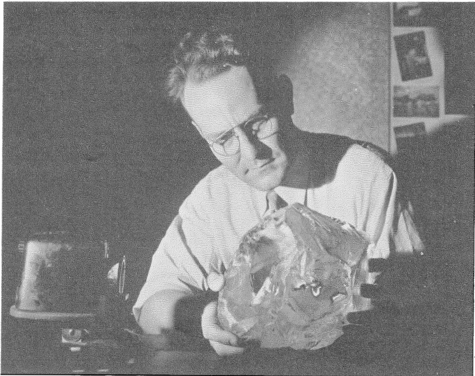
Fig. 7—Examining a Large Piece of Raw Quartz for Flaws Prior to Processing it at the Federal Telephone and Radio Corporation Crystal Laboratories in Newark, New Jersey.
