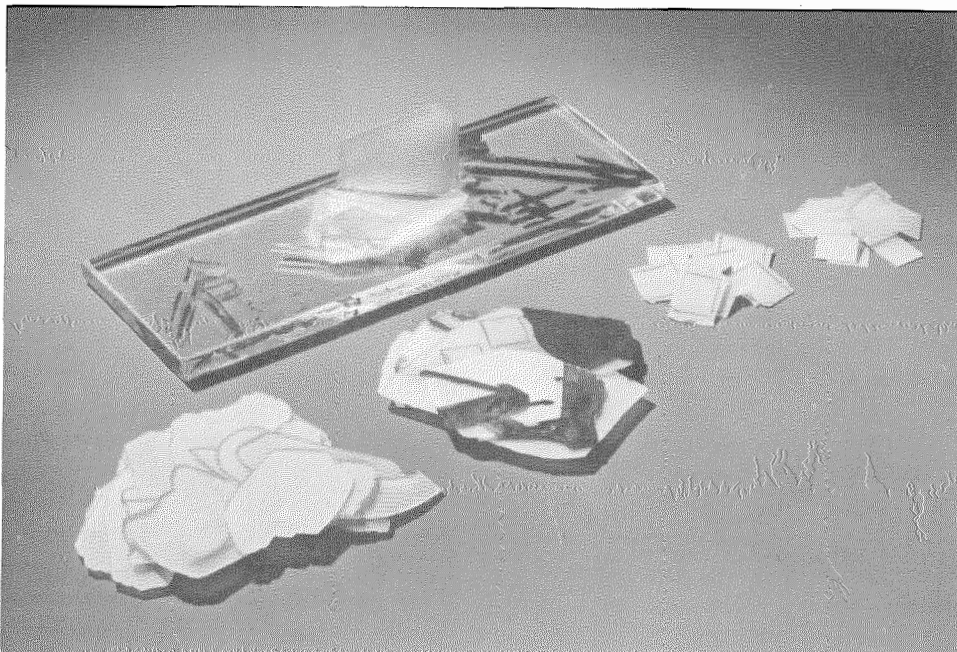
Fig. 9—Various Steps in Production from the Raw Crystal to the Finished Oscillator Blank are Shown Above. The Glass Block Illustrates how the Crystal Blanks are Sliced Out of Raw Quartz. On the Left are Rough Wafers Ready to be Classified. Next are Wafers with Twinned Portions and Flaws Blacked and with Framed Areas of Active Crystal Material. The Third Pile Shows the Diced or Roughed-Out Squares and the Last Pile the Finished Blanks.
