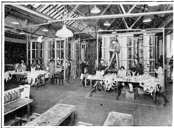
The Wiring Shop at Hendon, Showing the Wiring of Rotary Equipment. The Girls on the Front Benches are Preparing Ribbon Cables for Soldering.
