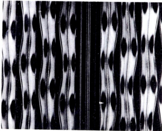
Fig. 6 Photomicrograph of single-channel 45-45 grooves.
