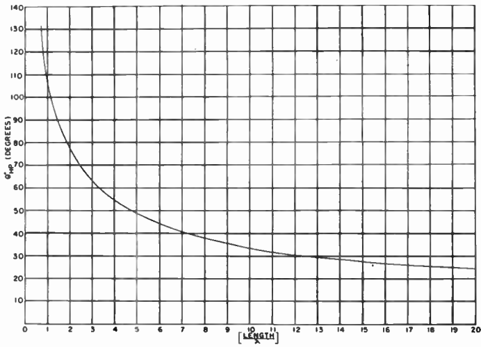
Fig. 20 Half-power beamwidth of a uniformly illuminated end-fire array as a function of array length
