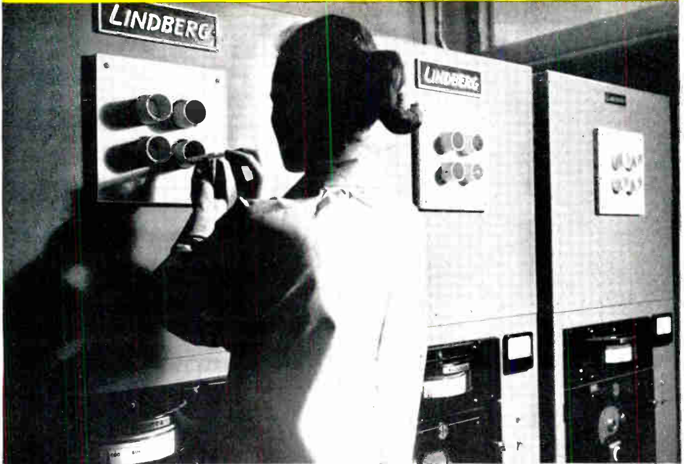
These Lindberg four-tube furnaces at Microwave Associates, Inc., provide maximum continuous operating temperature to 1371°C. (2500°F.). Chamber accommodates four 2" O. D. and has a uniformity of plus or minus 5.0°C.
