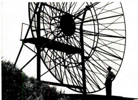
This giant transmitting antenna creates the beam for experimental antenna pattern measurements – part of the Hughes microwave research and development programs.
