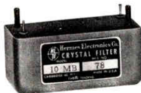
Hermes Crystal Filter, Model 10 MB, measures 2 3/8" long x 1" wide x 1 1/32" high.
