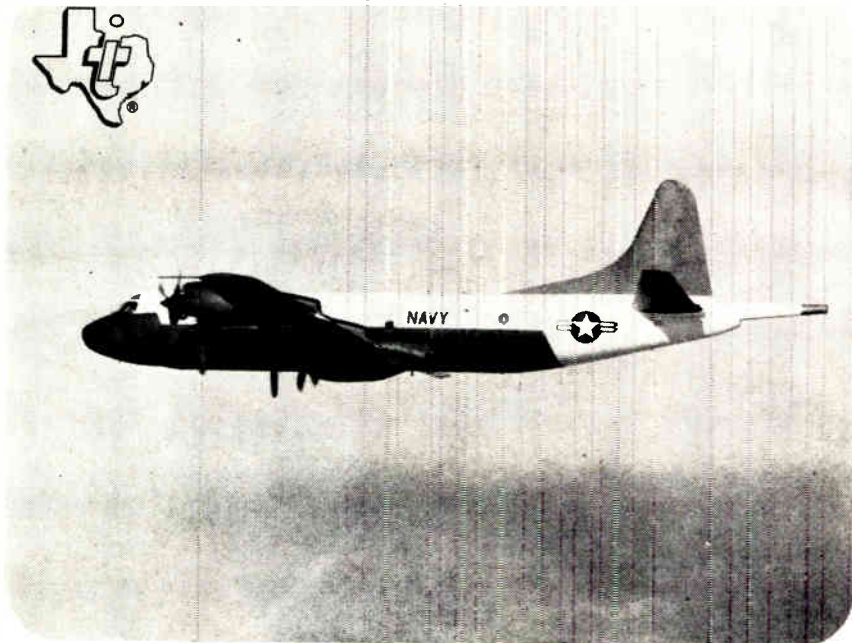
U. S. Navy P3V ELECTRA antisubmarine aircraft produced by Lockheed—equipped with TI-built AN/APS-80 surface search radar, AN/APA-125A indicator, AN/ASQ-8 magnetic anomaly detector and TD-239A intervalometer.
