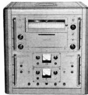
APR-20 rectangular antenna pattern recorder
