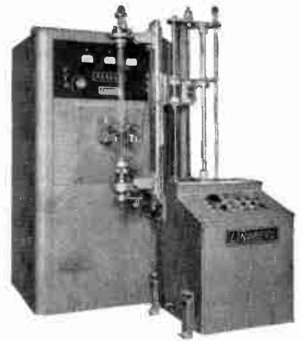
Vertical Floating Zone Scanner for accurate and precise production of hyper-pure semiconductor materials and metals.
