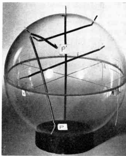
Fig. 1—Model of the Cayley-Klein representation of three-dimensional hyperbolic space showing the transformation of an impedance or a reflection coefficient through an ideal transformer.
