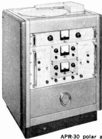
APR-30 polar antenna pattern recorder
