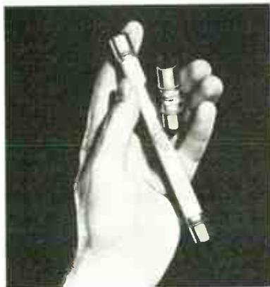
*This rectifier configuration was developed and introduced to industry by International Rectifier. The recent addition of high current types makes this the widest selection available. The current range is from 45 to 440ma. PIV voltages range from 1500 to 16,000 volts in standard types. With modification, the PIV can be increased to 20,000. On special order, 72,000 PIV units can be supplied. For complete technical data on these units . . .*
