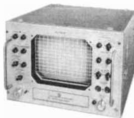
Applications include laboratory and production testing of band-pass filters, limiters, all types of amplifiers, television receivers, attenuators, discriminators and coaxial cables.
