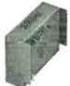
RF saturable inductor for sweep from 17 MC to 21 MC.
