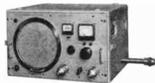
Applications: impedance measurements on semi-conductors, antennas, filters, receivers, amplifiers.
