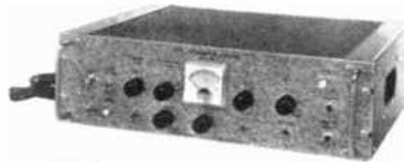
Used with an external crystal detector and directional coupler, the Model 700 can hold RF output from single frequency or swept microwave sources constant to  $\pm 0.1$  db at a fixed frequency.
